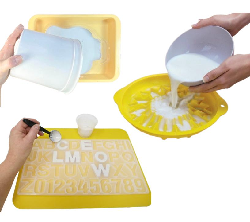
Whenever possible, pour plaster mixture starting in the deepest area to achieve an even flow across the surface of your mold. • Agitation or vibration of the filled mold will encourage dispersion of trapped air.
